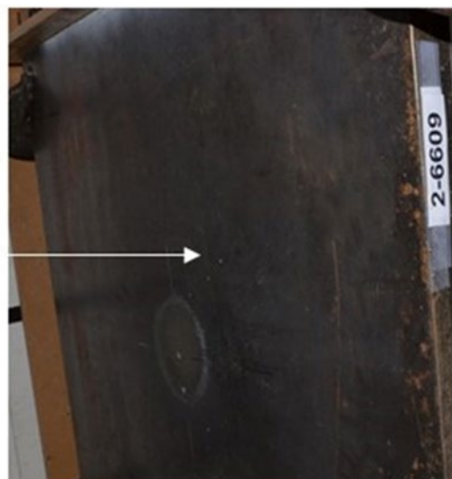
Figure 5. The top of the cell hit the stainless steel target at 90 degrees
